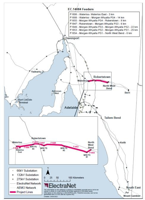
Figure 1 - Location of the line conductors identified for replacement
