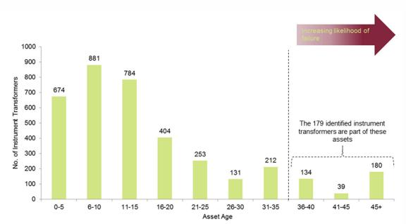
Figure 3 - Age profile of instrument transformers and increasing level of failure
