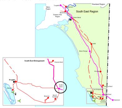
The two SVCs are critical in providing reliable power transfer by generating or absorbing reactive power in response to power system disturbances, thereby controlling voltage levels across the South Australian transmission network to maximise the transfer capability between South Australia and Victoria along the Heywood Interconnector.
