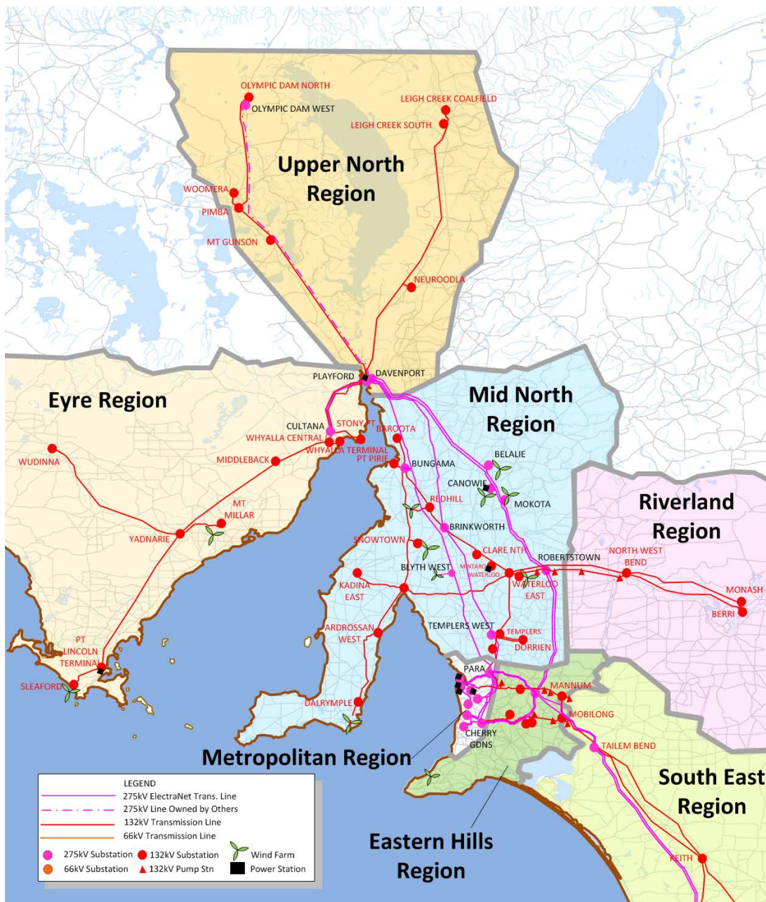
Figure 1: Geographical Diagram showing the existing network
