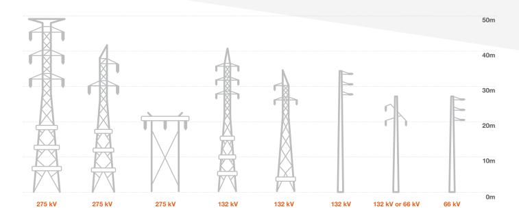
Overhead transmission lines are supported by a number of unique structure types, including steel lattice towers and masts, and several different pole designs, including a super-sized version of the well-known concrete and steel Stobie pole.
