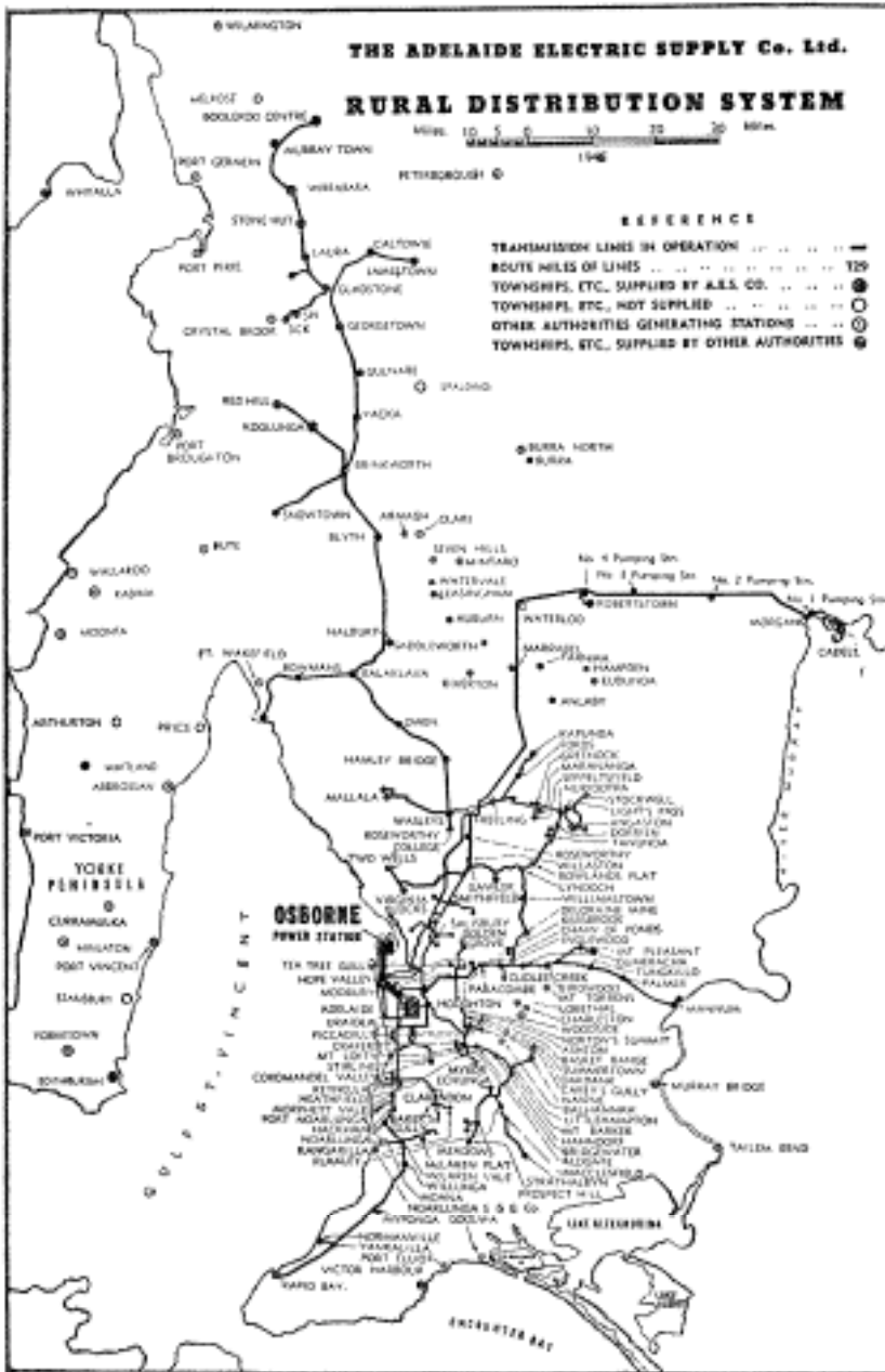
By DECEMBER 1946, THE TRANSMISSION SYSTEM HAD ALREADY MOVED INTO A LARGE NUMBER OF RURAL AREAS AND WAS PLANNED TO SPREAD AT A MUCH GREATER PACE AND INTENSITY. A COMPARISON WITH THE EARLIER MAP WILL CLEARLY SHOW THE DEVELOPMENTS ACHIEVED ADELECT MAGAZINE
