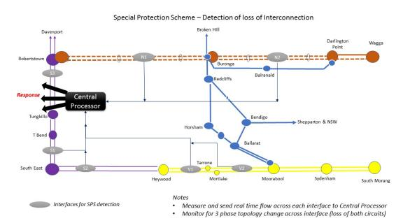
The scheme will require topology based signals along with power flows across each interface to be continuously transmitted to the central processor for real time pre-processing.
