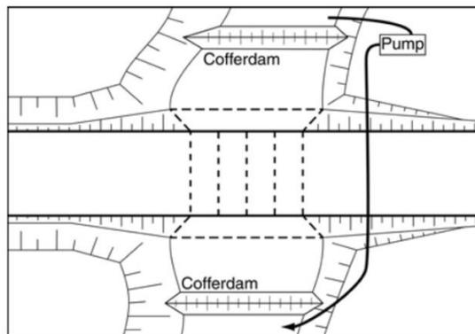
Figure 3: Cofferdam with bypass flow (Sourced from: Witheridge, 2017)
