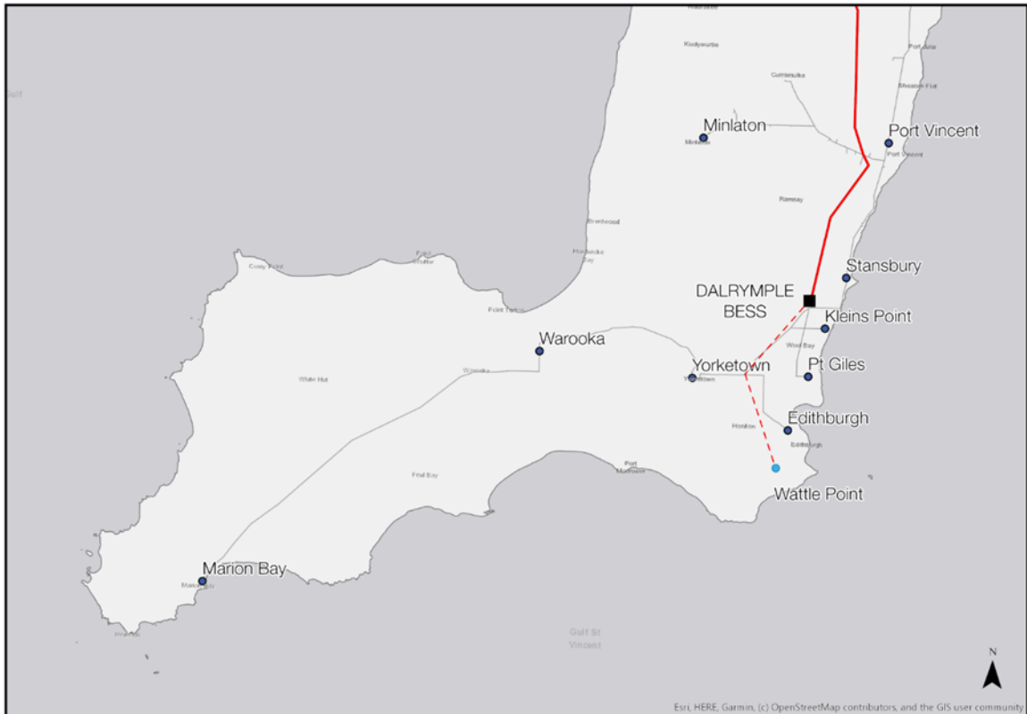
Figure 2-3: Region supported by the Dalrymple battery during an islanding event
