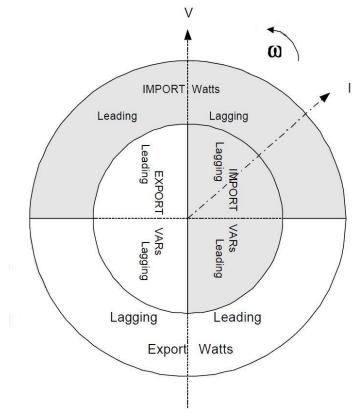
For the example shown in Figure 1, the current lags the voltage by 45°. The diagram indicates the condition is an *Import Lagging Watts* for this quadrant.
