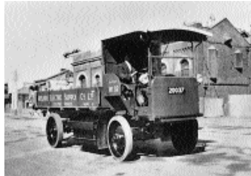
ELECTRIC TRUCK OUTSIDE AESCO'S BUILDING EAST TERRACE, ADELAIDE. IT WAS DRIVEN BY 'JACK' MARGITICH BETWEEN THE LATE 1920S AND EARLY 1930S. 'JACK' WORKED FOR ETSA FROM 1918 TO 1959. THIS ELECTRIC TRUCK HAD A SPEED OF 20 MPH, 3 TONS CAPACITY, A RANGE OF 40 TO 50 MILES AND WAS USED FOR DELIVERIES AROUND THE CITY, TO PORT ADELAIDE AND AS FAR NORTH AS SALISBURY. 'JACK'S' GRANDSON, BRIAN MARGITICH, WORKS AS A SYSTEM CONTROL OFFICER AT ELECTRANET SA IN THE SYSTEM CONTROL CENTRE ELECTRANET SA
